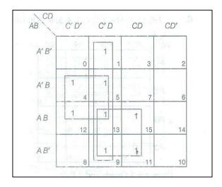
There are 3 Quads: Quad 1 ( $m_1 + m_5 + m_9 + m_{13}$ ) reduces to C'DQuad 2 ( $m_4 + m_5 + m_{12} + m_{13}$ ) reduces to BC'Quad 3 ( $m_9 + m_{11} + m_{13} + m_{15}$ ) reduces to ADHence, the final expression is: F(A, B, C) = C'D + BC' + AD
