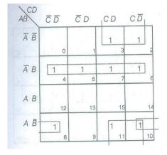
There are 2 Quads and 1 Pair: Quad 1 ( $m_4 + m_5 + m_6 + m_7$ ) reduces to  $\overline{AB}$ Quad 2 ( $m_2 + m_3 + m_{10} + m_{11}$ ) reduces to  $\overline{BC}$ Pair 1 ( $m_8 + m_{10}$ ) reduces to  $\overline{ABD}$ Hence, the final expression is:  $F(A, B, C, D) = \overline{AB} + \overline{BC} + A\overline{BD}$
