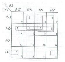
There are three Quads and 1 Pair: Quad 1 ( $m_1 + m_3 + m_5 + m_7$ ) reduces to P'SQuad 2 ( $m_4 + m_5 + m_6 + m_7$ ) reduces to P'QQuad 3 ( $m_2 + m_3 + m_6 + m_7$ ) reduces to P'RPair 1 ( $m_8 + m_{10}$ ) reduces to PQ'S' Hence, the final expression is: F(P, Q, R, S) = P'S + P'Q + P'R + PQ'S'
