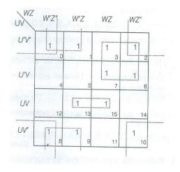
There are three Quads and 1 Pair: Quad 1 ( $m_0 + m_2 + m_8 + m_{10}$ ) reduces to VZQuad 2 ( $m_0 + m_1 + m_8 + m_9$ ) reduces to VWQuad 3 ( $m_2 + m_3 + m_6 + m_7$ ) reduces to UWPair 1 ( $m_{13} + m_{15}$ ) reduces to UVZHence, the final expression is: F(U, V, W, Z) = V'Z' + V'W' + U'W + UVZ
