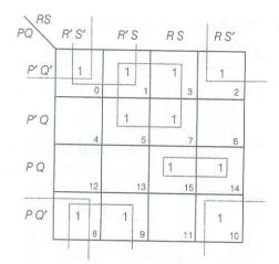
There are three Quads and 1 Pair: Quad 1 ( $m_0 + m_2 + m_8 + m_{10}$ ) reduces to  $\overline{QS}$ Quad 2 ( $m_1 + m_3 + m_5 + m_7$ ) reduces to  $\overline{PS}$ Quad 3 ( $m_0 + m_1 + m_8 + m_9$ ) reduces to  $\overline{QR}$ Pair 1 ( $m_{14} + m_{15}$ ) reduces to PQR Hence, the final expression is: H(P,Q,R,S) = Q'S' + P'S + Q'R' + PQR
