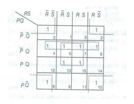
There are three Quads: Quad 1 ( $m_4 + m_5 + m_6 + m_7$ ) reduces to  $\overline{PQ}$ Quad 2 ( $m_5 + m_7 + m_{13} + m_{15}$ ) reduces to QSQuad 3 ( $m_0 + m_2 + m_8 + m_{10}$ ) reduces to QSHence, the final expression is:  $F(P, Q, R, S) = \overline{PQ} + QS + \overline{QS}$  4. Obtain the minimal form for the following boolean expression using Karnaugh's Map:
